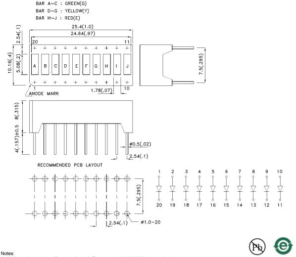
1. All dimensions are in millimeters (inches), Tolerance is ±0.25(0.01")unless otherwise noted.
